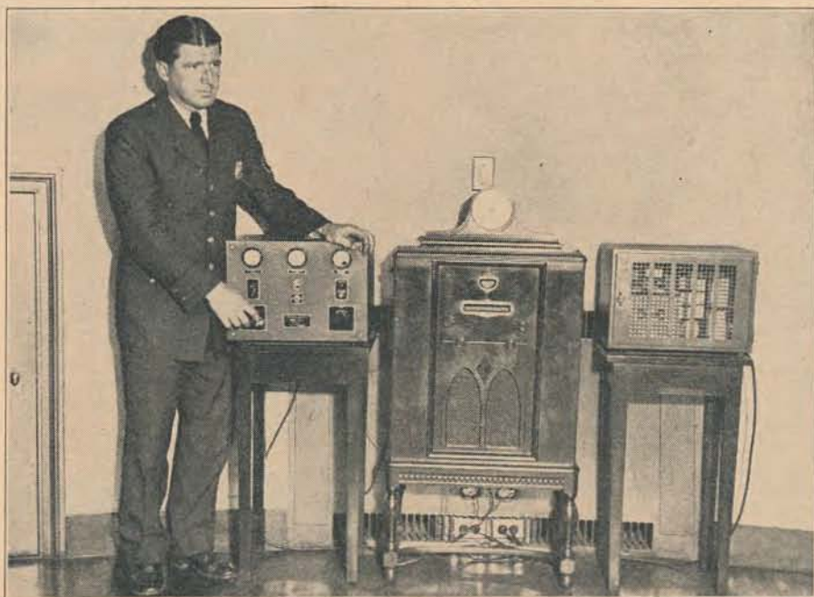
Dispatcher Carl Vollmer shown at the frequency monitor which checks wave lengths. This is a part of the New York police radio equipment
